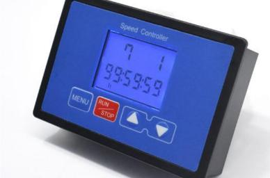
Set the number of motor start and stop cycles. Press the MENU key 8 times to enter the function 8 key surface. The
