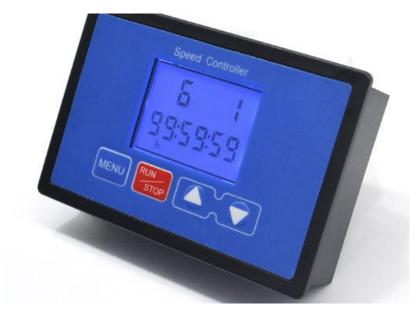
Motor stop time setting Press the MENU key 7 to enter the function 7 key surface. The default is 99 hours, 59 minutes, and 59 seconds. RUN / STOP key switching hours, minutes, and seconds
