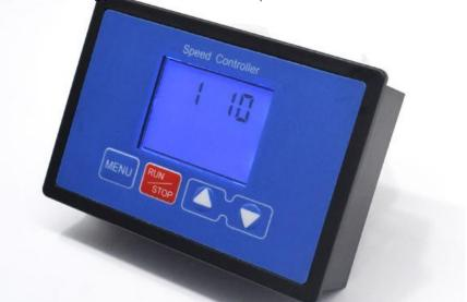
Slow stop time setting Press the MENU key 2 to enter the function 2 setting key surface Press the plus and minus keys to set the time Long press MENU to save and exit (10 for 1 second and 100 for 10 seconds)
