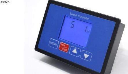
Motor running time setting Press the MENU key 6 to enter the function 6 key surface. The default is the maximum time 99 hours 59 minutes 59 seconds. RUN / STOP key switching hours minutes seconds Press plus, minus, hour, minute, and second. Press and hold MENU to save and exit.
