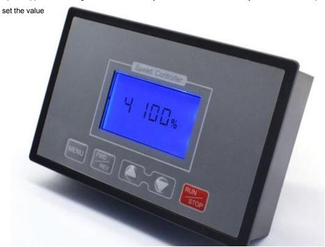
Acceleration / deceleration value setting Press the MENU key 6 to enter the function 5 key surface Press the plus / minus key to switch Press RUN / STOP to save and exit
