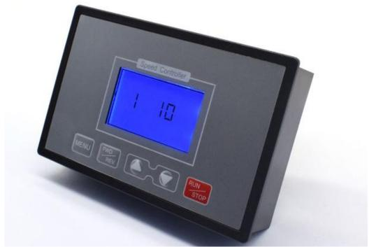
Slow stop time setting Press the MENU key 3 to enter the function 2 setting key surface Press the plus and minus keys to set the time Press RUN / STOP to save and exit (10 is 1 second and 100 is 10 seconds)
