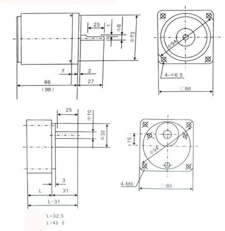
Tip: If the reduction ratio is larger, L (height) in the image is larger.
