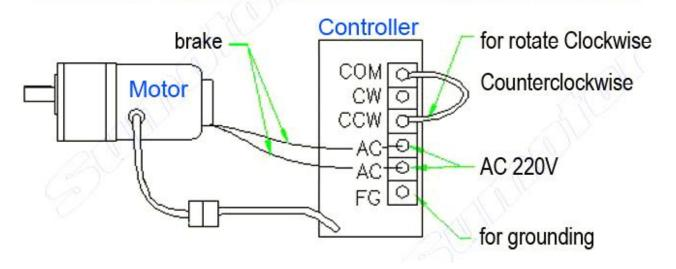
Brake Fundamental: When switch on brake, the resistance will disappear. When switch off brake , the brake will resist to motor rotation. When all circuit is closed, the brake will not affect the motor, at the instant of circuit open, brake will resist to stop motor instantly.
