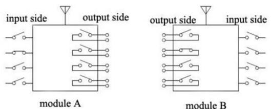
Also in this mode, the slave will regularly send inquiries to the master for link status. If no acknowledged signal come to the master, the alarm LED will light on, after the inquiry time is over and all the output relays will be resumed open.
