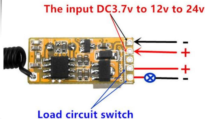
The input DC3.7v to 12v to 24v
