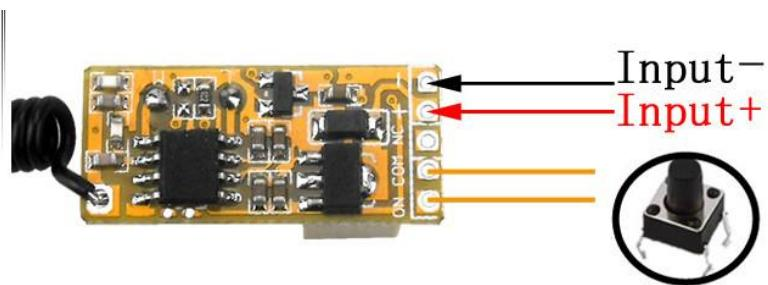
Input DC 3.7V to 24V Output 0V Switching Value
