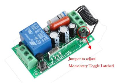
Momentary---Jumper on "M&G" Toggle--Jumper on "G&T" Latched-Jumper on 1 Pin or Take away Jumper
