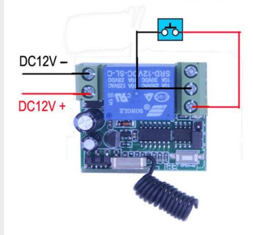
Jumper: 1&2 working way Latched Jumper: 2&3 working way Toggle Jumper non-occupation working way : Momentary To change Toggle . Latched . Momentary
