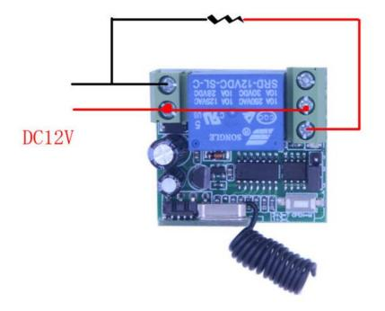
Entrance guard control wiring diagram
