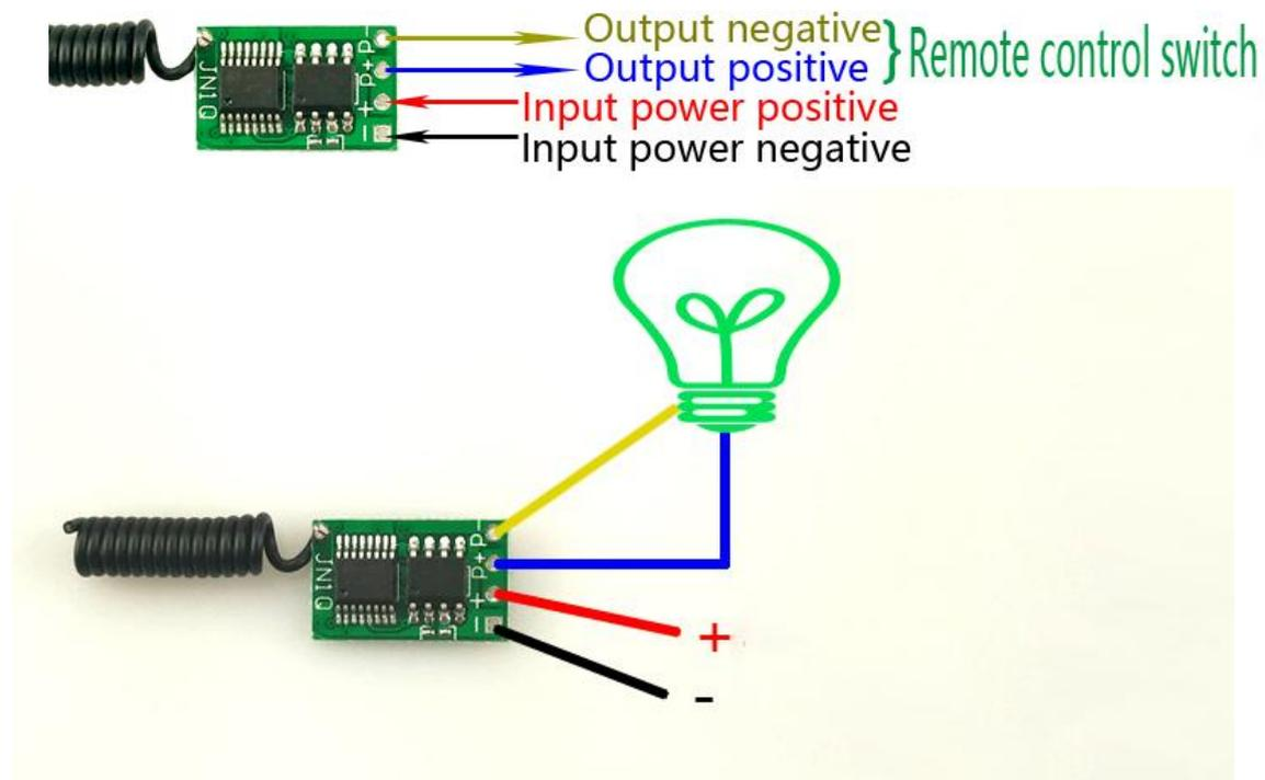
Control range: 3v to 24v ( 10 watts )
