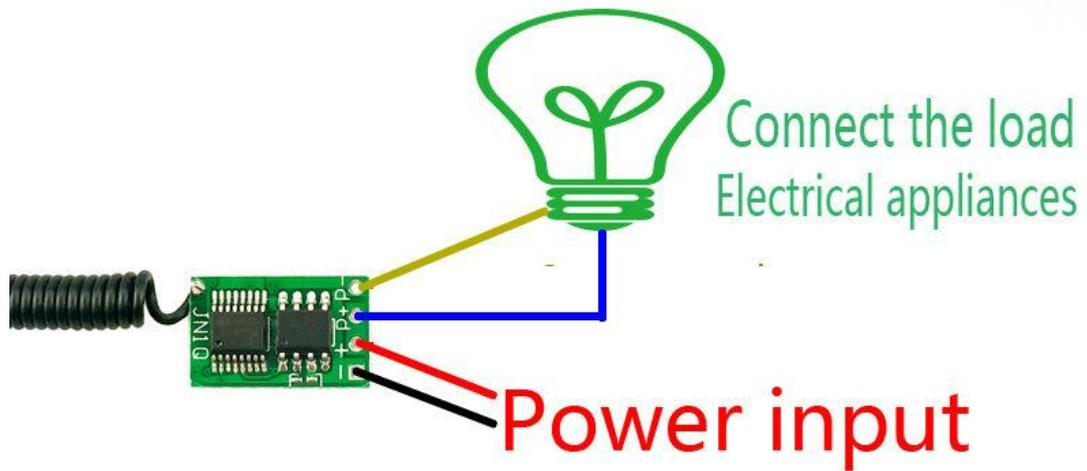
Input supply voltage → Remote on = The output voltage
