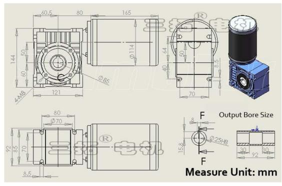
This motor Output power through Bore, need addition shaft, we have shaft suitable on sale, Bore Diameter is looks like the drawing.
