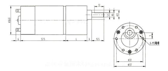
**Attention:** The baby is a big torque, high power motor and the starting current is a little large, 6V starting flow is around 3A, 12V starting current is about 6A, the starting current will return to normal 1-2A when starting, so you need select high power supply, 6V need be above 5A while 12v need be above 10A. otherwise it can not start the motor!!
